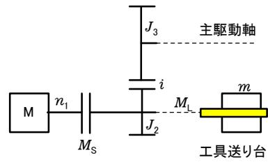
被動側の質量慣性モーメント:  $J_{2\text{等価}}=J_2+\frac{J_3}{i^2}+m\left(\frac{v}{\omega_{10}}\right)^2=0.04\text{kg}\cdot\text{m}^2+\frac{0.5\text{kg}\cdot\text{m}^2}{2.8^2}+800\text{kg}\times\left(\frac{1\text{m}/\text{s}}{150\text{s}^{-1}}\right)^2=0.14\text{kg}\cdot\text{m}^2$
